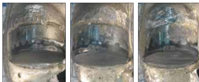
♦♦♦ Fig 8 Wear on new cutters after 8.2 km of sliding distance
