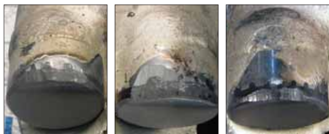
♦♦♦ Fig 7 Wear on original cutters after 8.2 km of sliding distance
